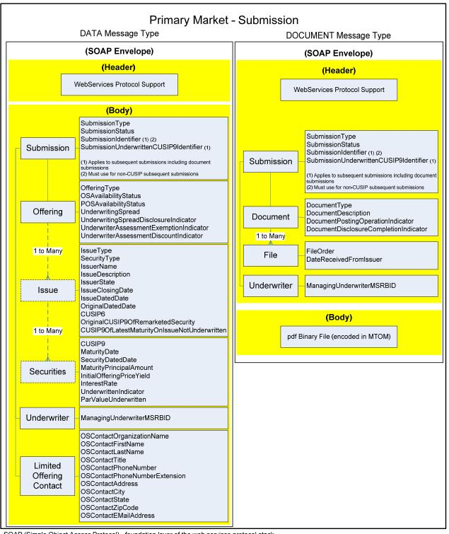
SOAP (Simple Object Access Protocol) - foundation layer of the web services protocol stack MTOM (SOAP Message Transmission Optimization Mechanism) - a method of efficiently sending binary data to and from web services
